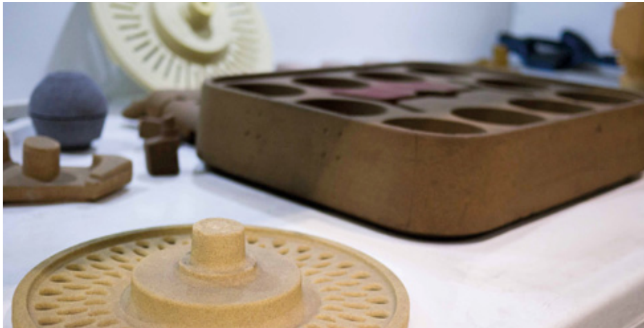
The core shooters from Laempe Mössner Sinto produce different sand cores for metal casting
